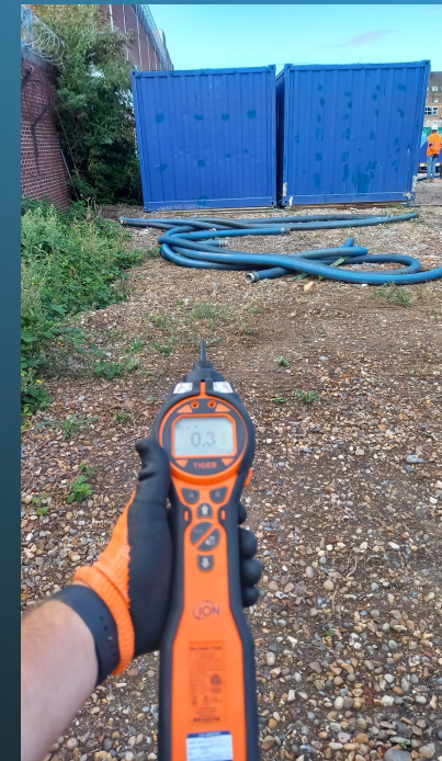
Real time environmental monitor in place on boundary to site, near to closest residential receptors.
